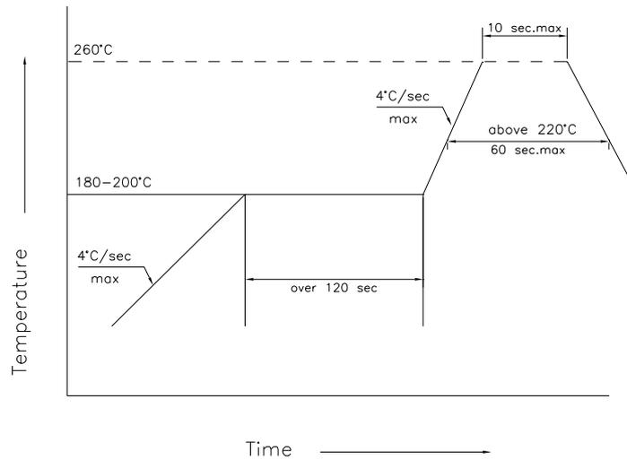
1. Reflow soldering should not be done more than two times.
